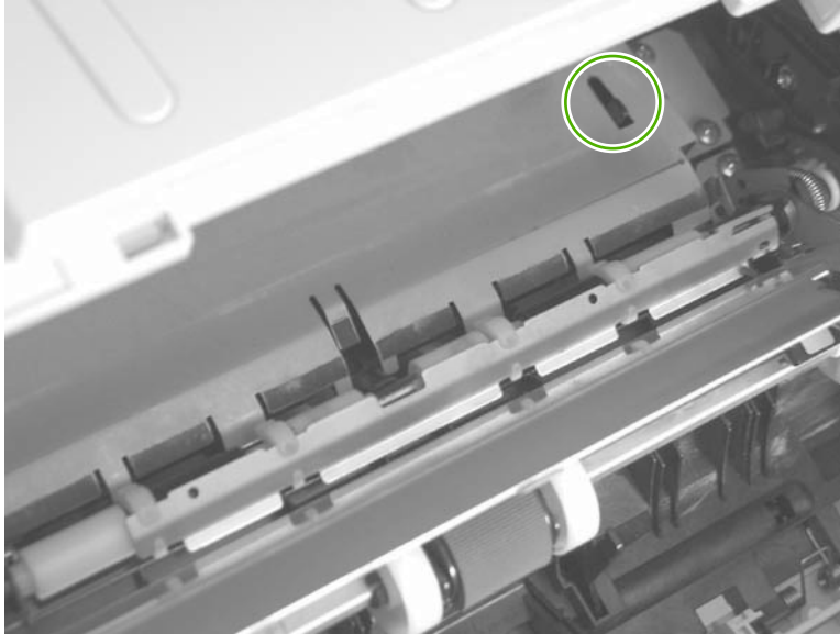
Figure 3-6 Test the media width sensor
