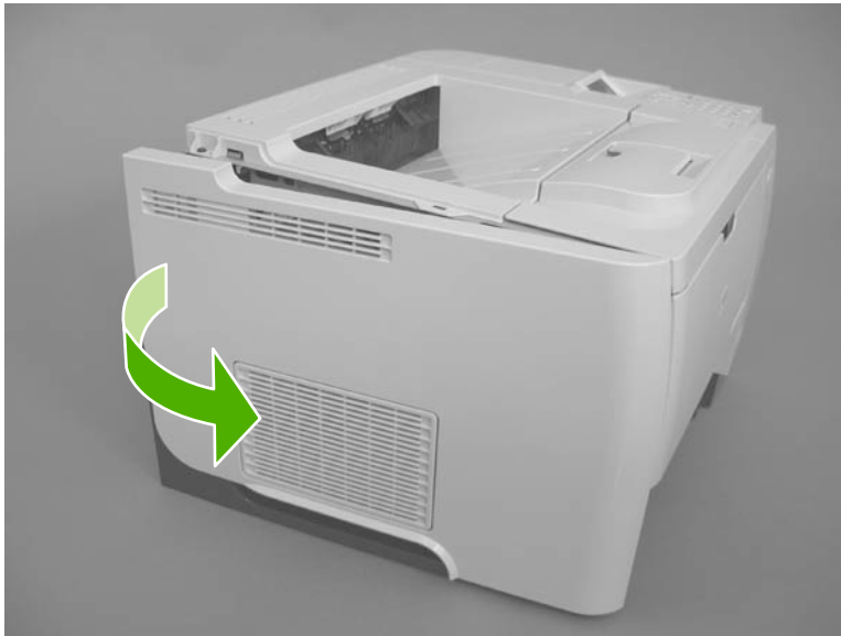
Figure 2-31 Remove the left cover (4 of 4)
