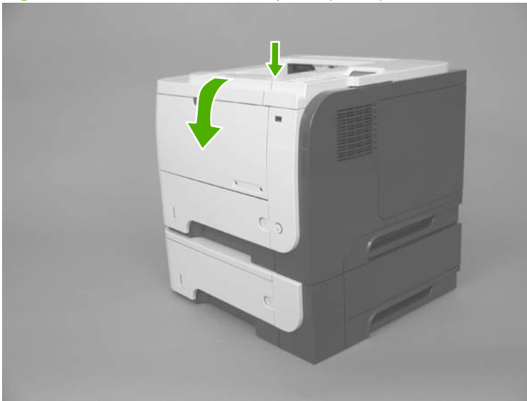
Figure 2-42 Remove the control panel (1 of 4)
