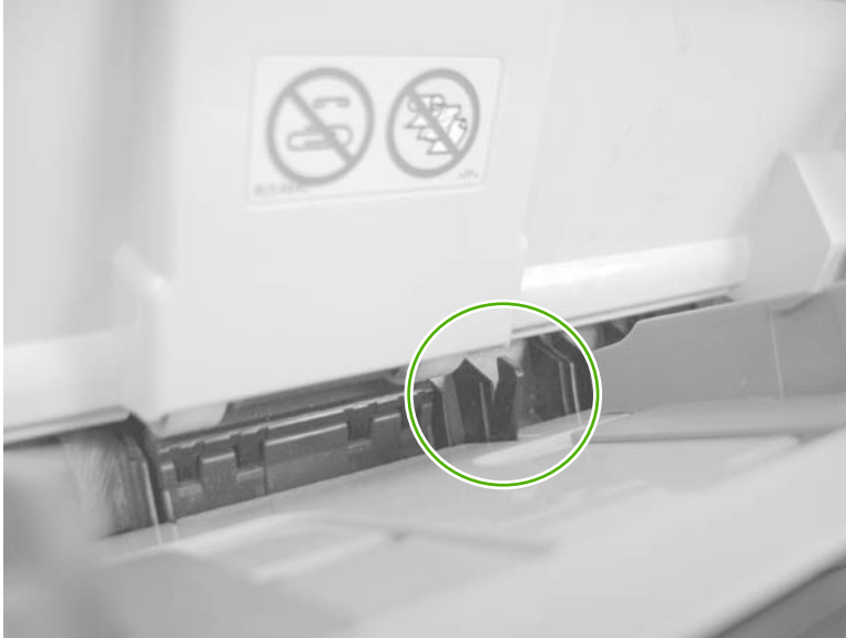
Figure 3-14 Test the Tray 1 (multipurpose tray) media-presence sensor
