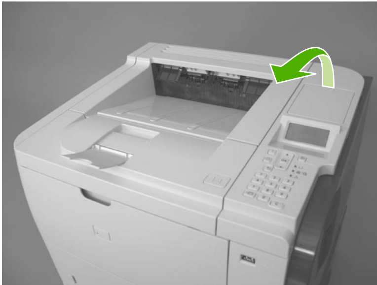
Figure 2-8 Remove the sub cover
