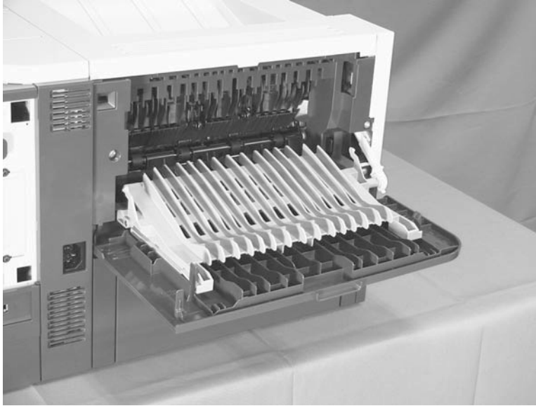
Figure 3-13 Test the face-up detect sensor (2 of 2)
