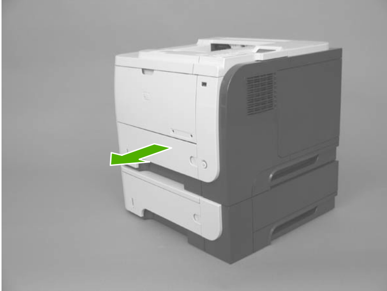
Figure 2-6 Remove the tray cassette (1 of 2)
